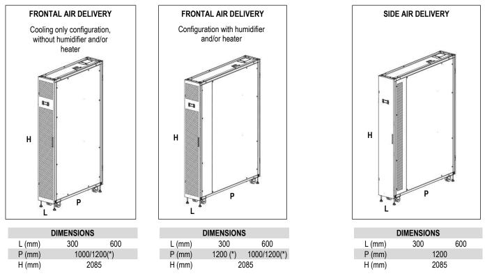
(\*) Increased frame dimensions for in-row version with frontal air delivery. Optional mandatory for in-row version with frontal air delivery with Humidifier (optional) and/or electric heater (optional).
