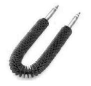
Tubular electric heater with steel fins. The optional is installed downstream the main cooling coil. Electric heaters have a three-stage control. The optional accessory requires increased frame dimensions (optional) for in-row version with frontal air
